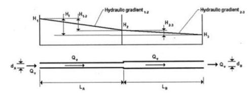
In the pipe network consisting of pipes of various diameters in series with each other, the same total flow Q must pass through each of the pipes in turn. The velocity in each section of the pipe will very depending on the diameter, so the head loss will very. Where pipe lengths differ, the head loss also be affected. A flow Q through the series network will have a total head loss  $H_f$  along the whole length which is the sum of the losses in each of the individual pipes.
