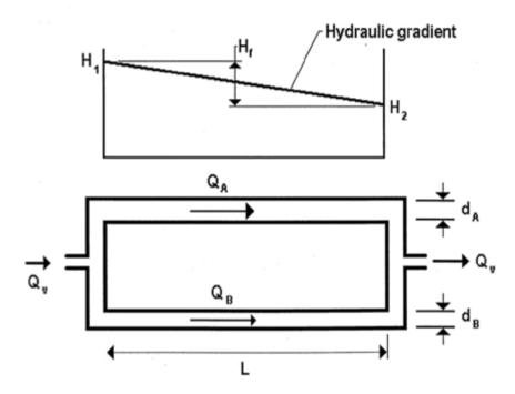
In the pipe network consisting of pipes of various diameters in parallel with each other, the pressure in the common mainflods, at the junction of the pipes, must be the same for all the pipes. The total flow  $Q_V$  therefore disturbs itself between the individual pipes in accordance with the controlling end pressure and:
