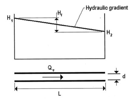
Any pipeline of diameter (D) and length (L) carrying a flow rate (Q) within a network will have a head loss along its length. This head loss is largely the result of pipe friction and:
