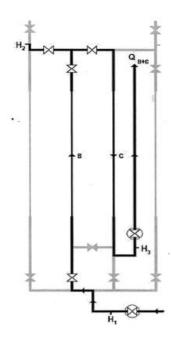
Repeat these measurements with the network of pipe configured for two alternative pipes in series then three pipes in series as shown in the diagram below:
