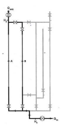
Repeat these measurements with the network of pipe configured for three pipes in parallel then four pipes in parallel as shown in the diagram below:
